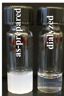
Fig. 3-6 Comparison between the appearance of as-prepared and dialyzed LaPO 4 core NPs suspensions.
